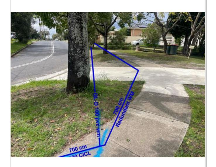
Redundant water main quality QL-C. 100 PVC water main located with GPR, QL-C.
