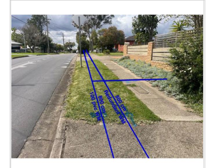
Redundant water main QL-C 100 PVC water main located with GPR, QL-C.
