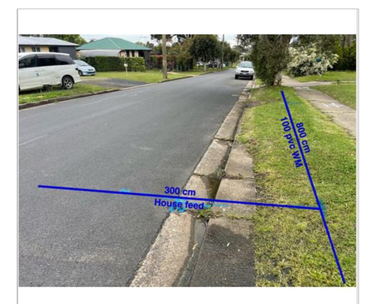
Redundant water main quality QL-C. 100 PVC water main located with GPR, QL-C.
